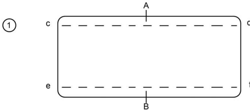
Calculate the distance between the lowest and uppermost heating strip, and mark two horizontal, parallel lines on the glass (cd and ef on diagram 1). Note, these must be at least 12" (305mm) apart). Mark a vertical line at each end (gh and ij on diagram 2)
