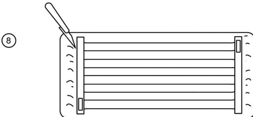
Remove the transparent film from the heating strips.
