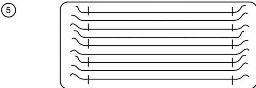
Stick the double sided tape to the inside of the glass along the lines gh and ij (as per Diagram 2), leaving a gap of at least 10mm between the strip and the window rubber.
