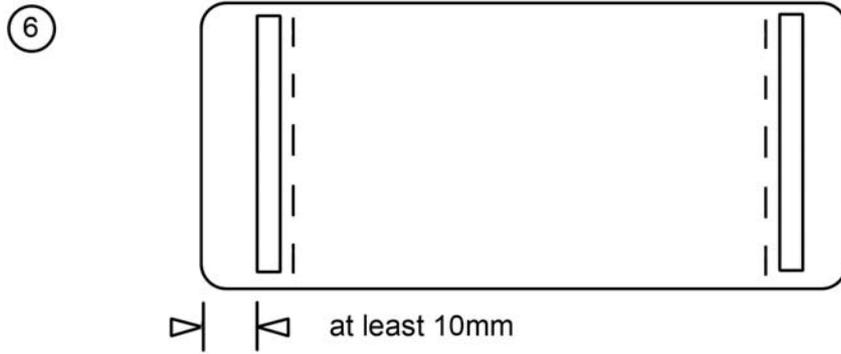
Lay the ends of the heater strip over the self adhesive strip and press the conductor strips firmly over the top, the conductor strips must cover all heating strips, and be mounted such that one of the wiring connectors is at the top and the other at the bottom.
